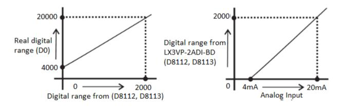
3) Suppose the user needs 4000-20000, and save in D0, so D0=8\*(D8112 or D8113) +4000, the program as following shows.
